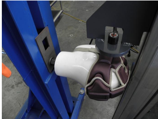
FIG.2C HEADSAVER HELMET LATERAL IMPACT TEST SET-UP
